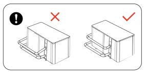
2.1.2. In order to guarantee the heating efficiency, the water pipe length should be  $\leq 10m$  between the pool and the heat pump.
