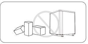
1.4.4. Don't put anything into inlet or outlet, or the efficiency of the heat pump will be reduced or even stopped.
