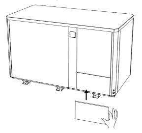
③ Fix the internal panel by two screws
