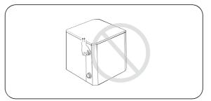
1.4.3. Don't put obstacles before the air inlet and outlet of the heat pump.
